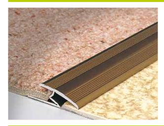
The multipurpose, grooved CARPETEC MP profile bends to clamp carpet flooring at different elevations. They may be used to join two types of carpeting or as edge profiles.
